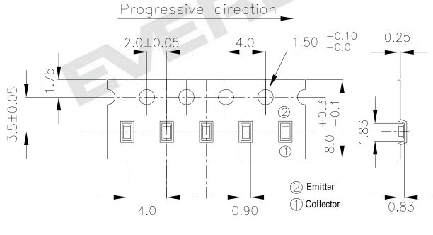
Unit: mm Tolerance: ±0.1mm
