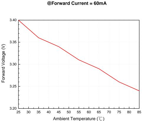
Forward Voltage vs. Ambient Temperature @Forward Current = 60mA
