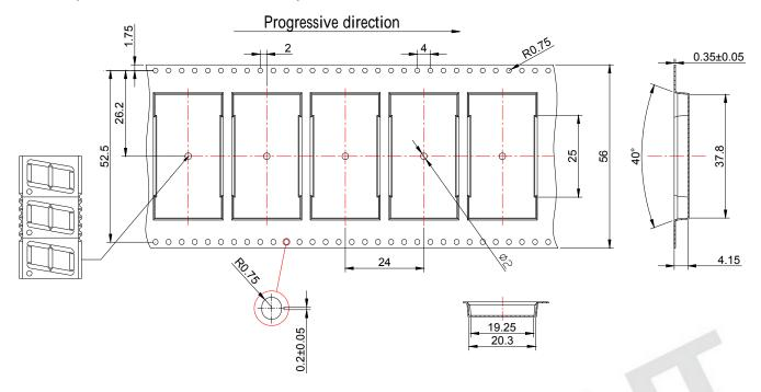
Note: Tolerances unless mentioned ±0.25mm. Unit = mm
