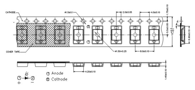
**Note:** The tolerances unless mentioned are ±0.1 mm, unit: mm.
