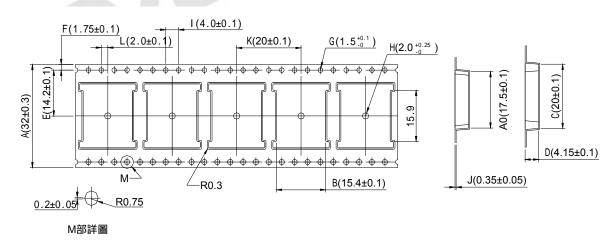
Note: Tolerances unless mentioned ±0.25mm. Unit = mm
