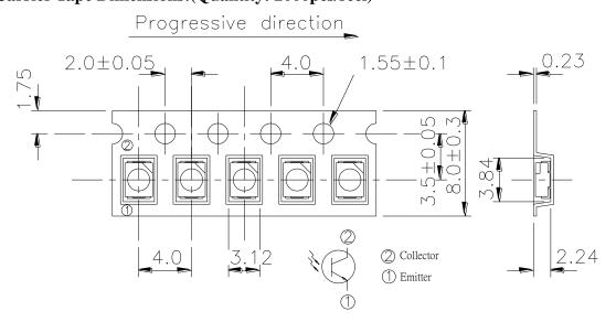
TOLERANCES UNLESS DIMENSION±0.1 ANGLE±0.5 UNIT:mm
