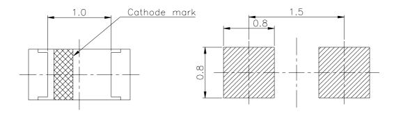
**Note:** The tolerances unless mentioned are  $\pm 0.1$ , unit = mm.
