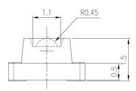
For reflow soldering (propose)
