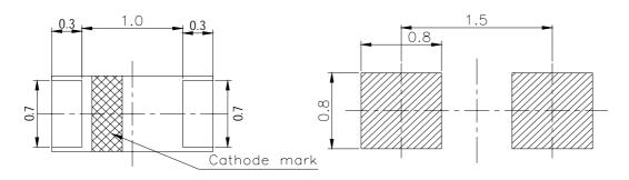
**Note:** The tolerances unless mentioned is  $\pm 0.1$ mm, Unit = mm
