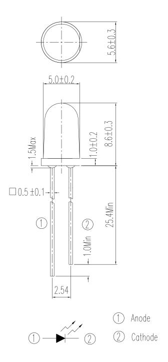
Note: Tolerances unless dimensions ±0.25mm
