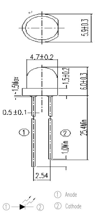
Note: Tolerances unless dimensions ±0.25mm
