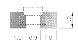
For Reflow Soldering (propose)
