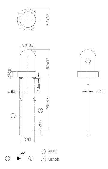
Note: Tolerances unless dimensions ±0.25mm
