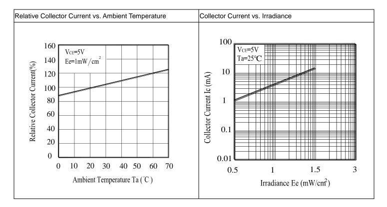
DATASHEET 5mm Phototransistor PT333-3C
