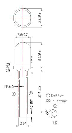
Note: Tolerances unless dimensions ±0.25mm
