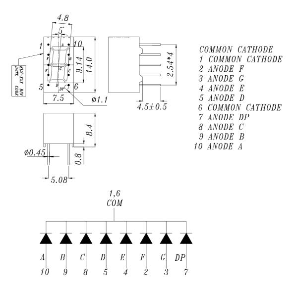
Note: Tolerances unless mentioned  $\pm 0.25$ mm. Unit = mm
