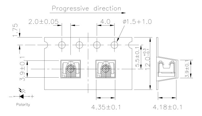
**Note:** Tolerance unless mentioned is  $\pm 0.1$ mm, unit = mm.
