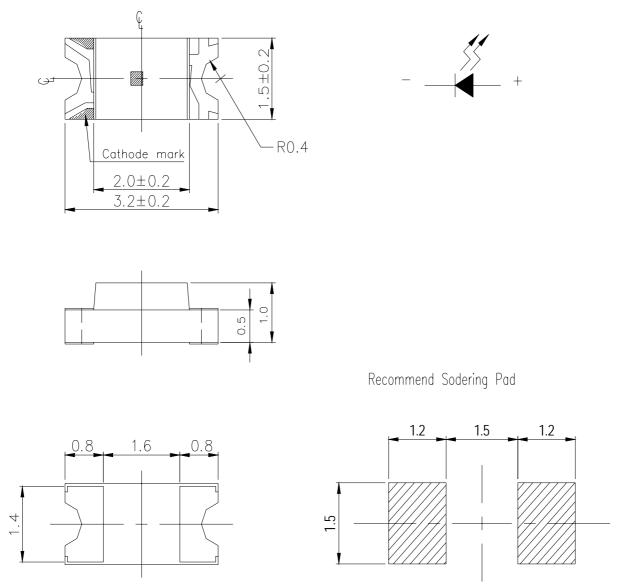
**Note:** Tolerances Unless Dimension  $\pm 0.1$ mm, Unit = mm
