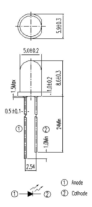
Note: Tolerances unless dimensions ±0.25mm
