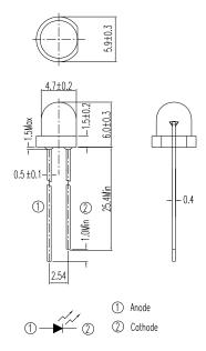
Note: Tolerances unless dimensions ±0.25mm
