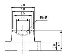
For reflow soldering (propose)
