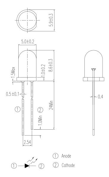
Note: Tolerances unless dimensions ±0.25mm
