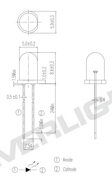
Note: Tolerances unless dimensions ±0.25mm
