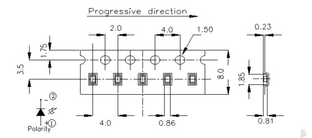
Note: The tolerances unless mentioned is ±0.1mm ,Unit = mm
