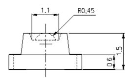
For reflow soldering (propose)
