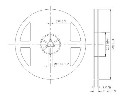
**Note:** The tolerances unless mentioned are  $\pm 0.1$ , Unit = mm.
