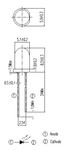
Note: Tolerances unless dimensions ±0.25mm
