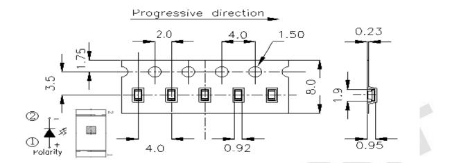
**Note:** The tolerances unless mentioned is  $\pm 0.1$  mm, Unit = mm
