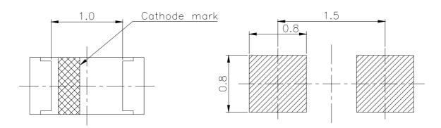
**Note:** The tolerances unless mentioned is  $\pm 0.1$ , Unit = mm
