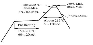
3.2 Reflow soldering should not be done more than two times.
