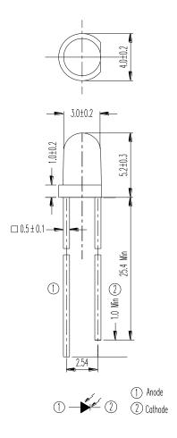
Note: Tolerances unless dimensions ±0.25mm
