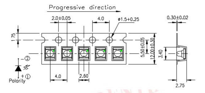
**Note:** The tolerances unless mentioned is  $\pm 0.1 \text{mm}$ , Unit = mm
