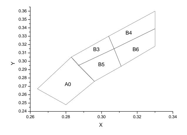
\*The C.I.E. 1931 chromaticity diagram ( Tolerance  $\pm 0.01$ ).
