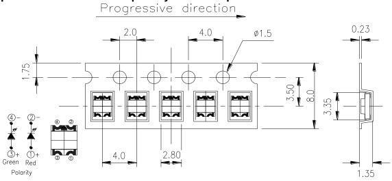
**Note:** The tolerances unless mentioned is  $\pm 0.1$ mm ,Unit = mm **Moisture Resistant Packaging**
