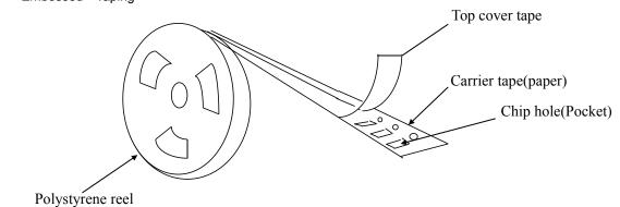
Dimensions of embossed taping for 0805~1812 type 送带孔 Feeding hole
