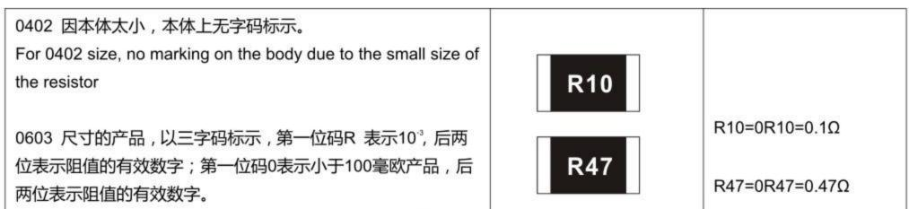
For 0603 size, use three digitals to declare resistance. The first letter 'R'denotes 10-3, The other two digitals declare resistance ; The first letter '0'means less than 100 mohm products, The other two digitals declare resistance.
