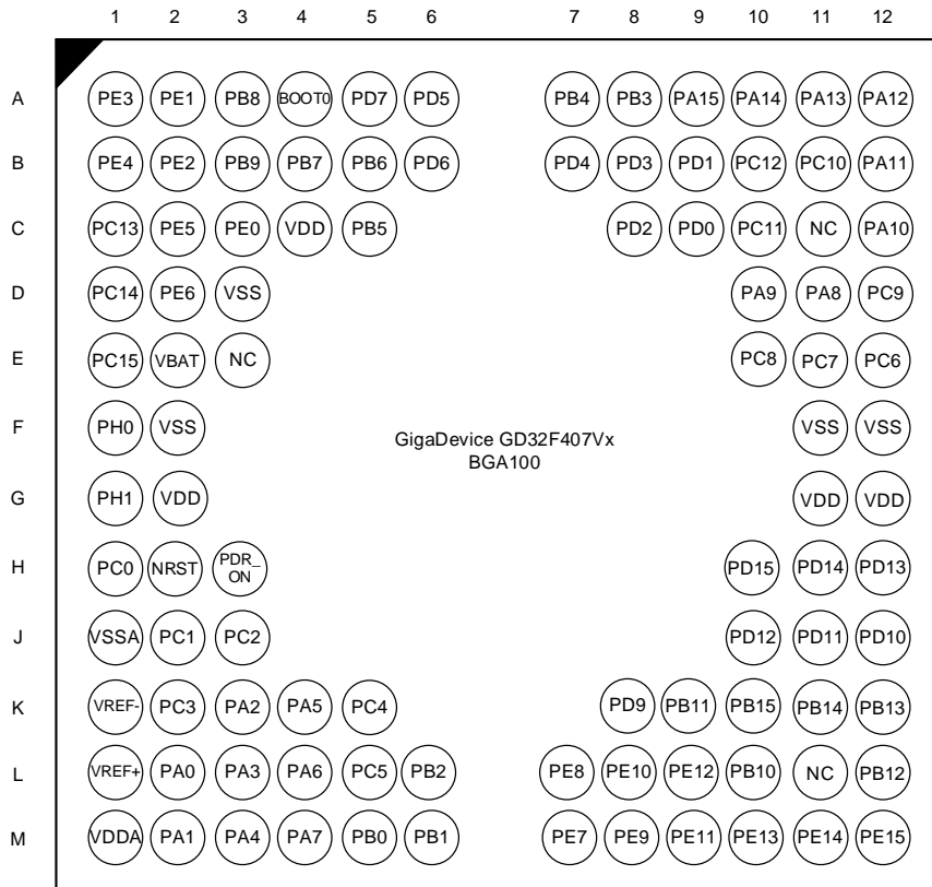
Figure 3. GD32F407Vx BGA100 pinouts
