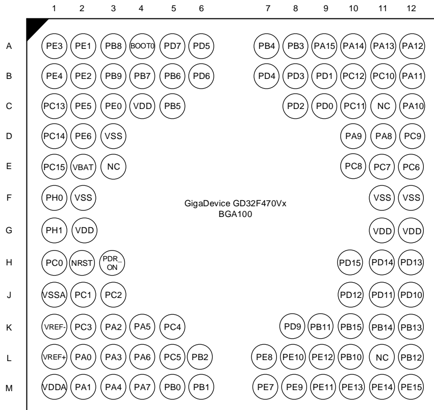
Figure 2-4. GD32F470Vx BGA100 pinouts
