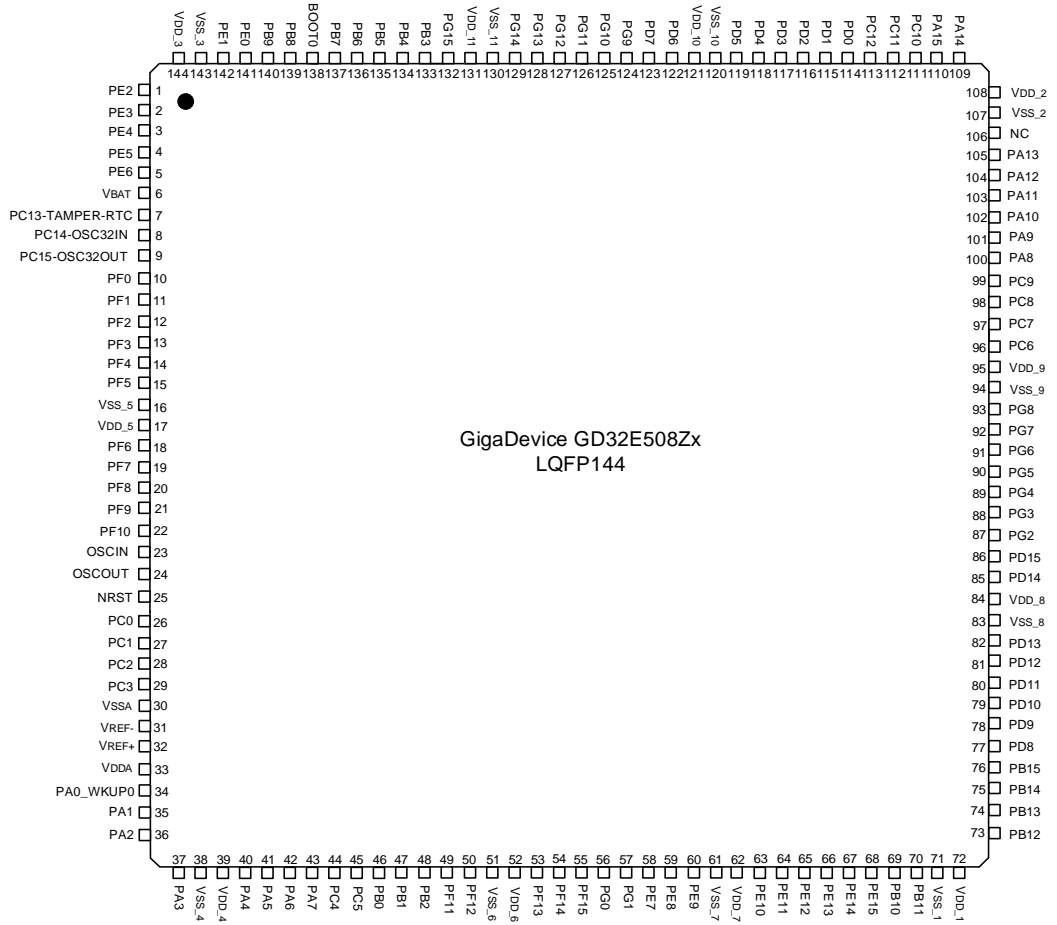
Figure 2-2. GD32E508Zx LQFP144 pinouts
