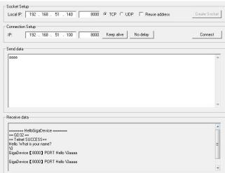
Using Network assistant software, configure the pc side to tcp server, using 1026 port, and when send something through the assistant, users can see the echo reply from the client:
