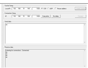
Using Network assistant software, configure to use udp protocol, using 1025 port, and when send something through the assistant, users can see the echo reply from the board:
