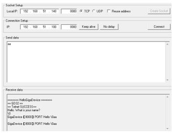
Using Network assistant software, configure the pc side to tcp server, using 1026 port, press the Tamper key, and when send something through the assistant, users can see the echo reply from the client:
