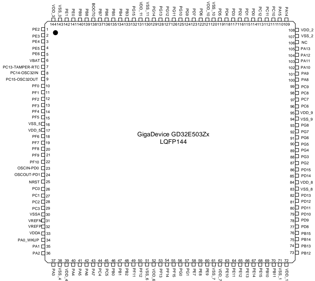
Figure 2-2. GD32E503Zx LQFP144 pinouts
