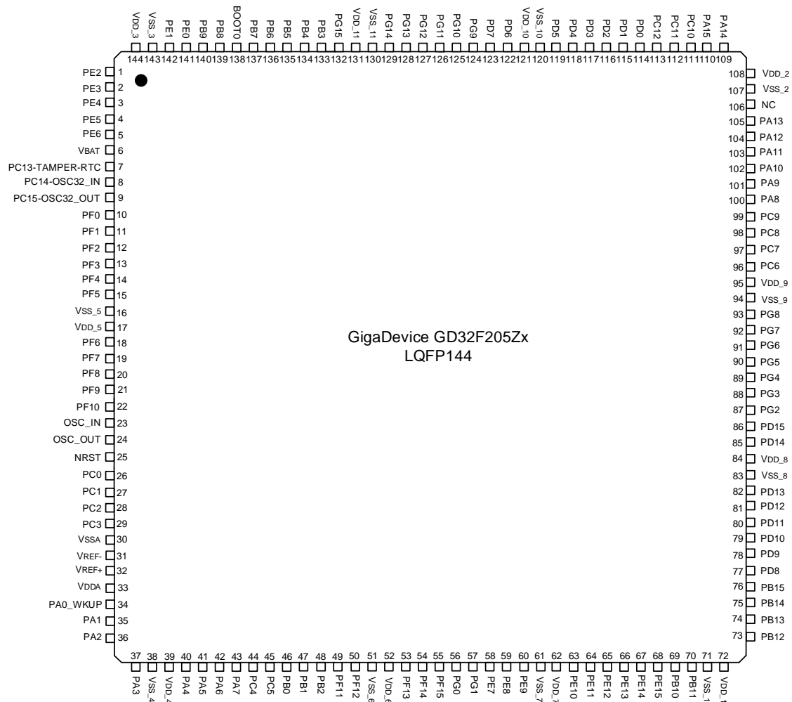
Figure 2. GD32F205Zx LQFP144 pinouts
