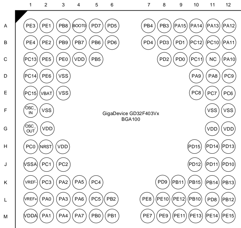
Figure 5. GD32F403Vx BGA100 pinouts
