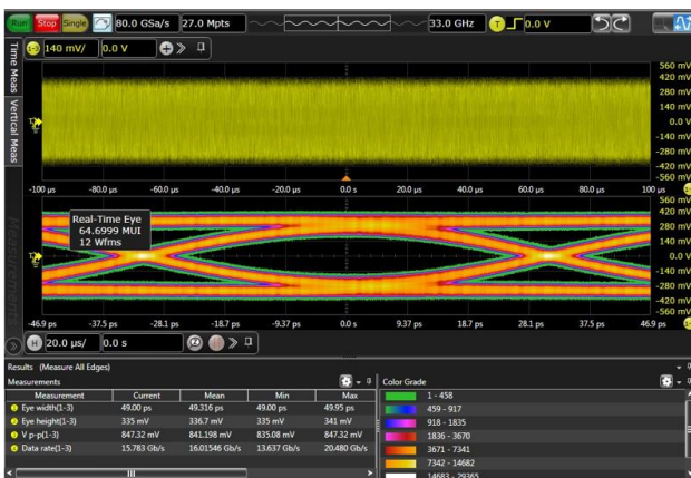
Figure 15, PCIe4.0 Eye diagram test, 16Gbps, Vpp=1V, With Device
