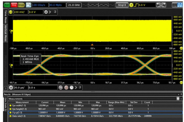
Figure 10, PCIe3.0 Eye diagram test, 8Gbps, V_{pp}=1.3V , No Device through Path
