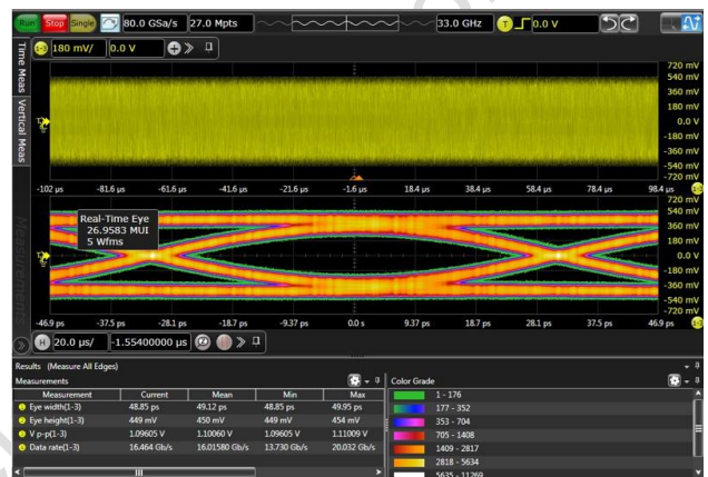
Figure 16, PCIe4.0 Eye diagram test, 16Gbps, Vpp=1.3V, With Device
