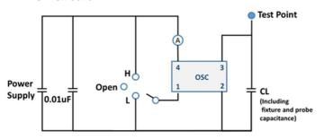
CL = Include jig & probe capacitance (Refer to 4)
