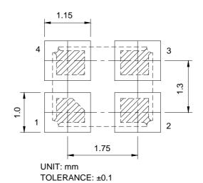
Chamfer index mark depends on the ceramic base supplier
