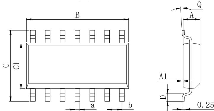
**Dimensions In Millimeters(SOP-14)**
