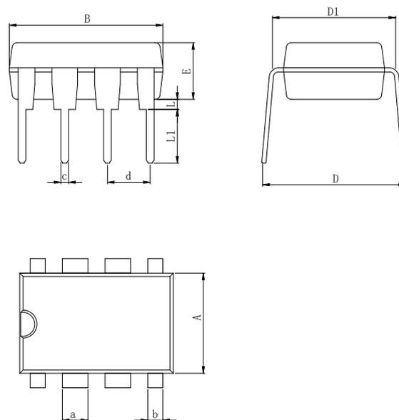
**Dimensions In Millimeters(DIP8)**
