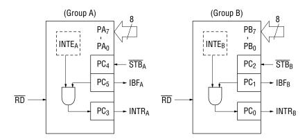
**Note:** Although belonging to group B, PC<sub>3</sub> operates as the control signal of group A functionally.
