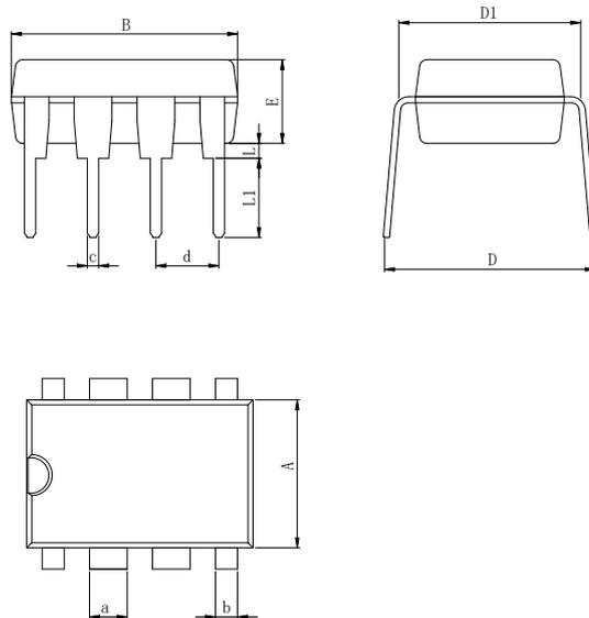
Dimensions In Millimeters(DIP-8)
