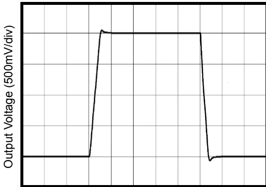
Non-Inverting Large-Signal Step Response
